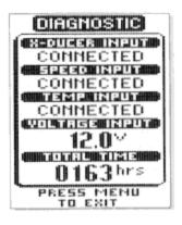
If you are using multiple transducers, switch between transducers to confirm the connections for each.
